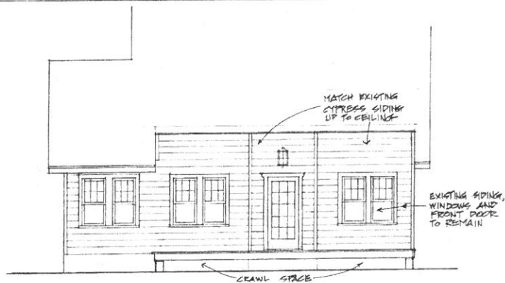
FRONT PORCH ELEVATION SC: 1/4"
