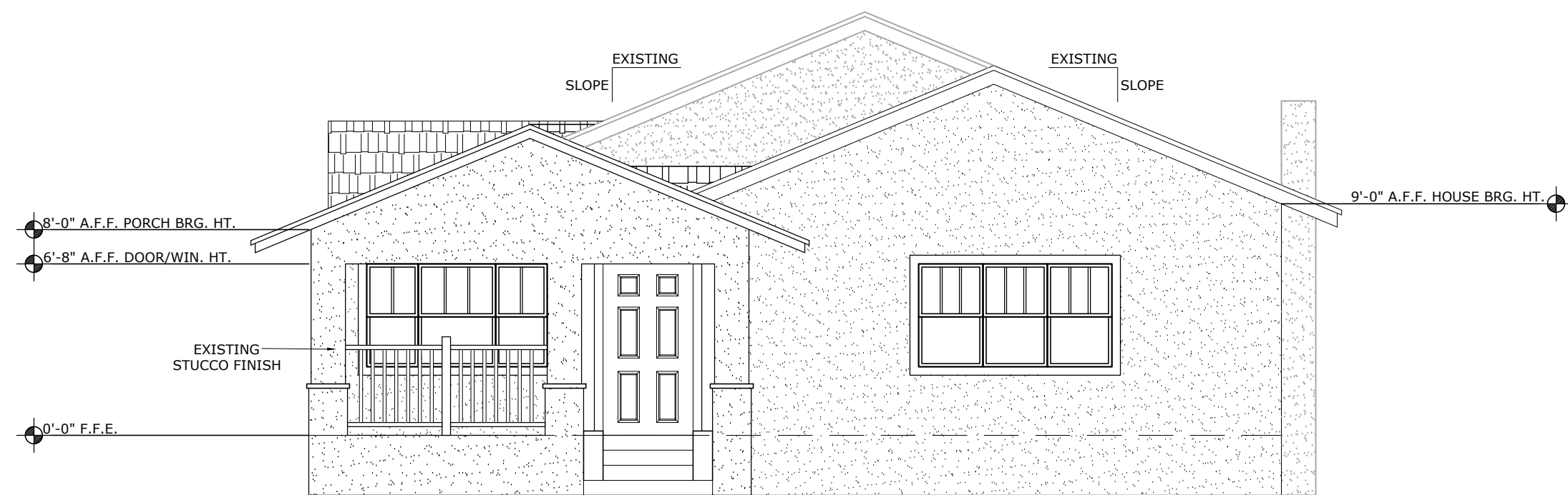
FRONT ELEVATION SCALE: 3/16" = 1'-0" (FIELD VERIFY ALL DIMENSIONS)
