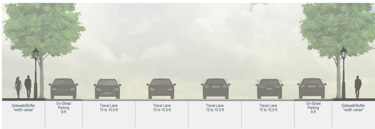
FIGURE 4: EXISTING TYPICAL SECTION OF ORANGE AVENUE
