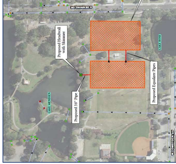
Alternative 1 – Exfiltration Basin Decrease in peak stage (100 yr): 0.26 ft Estimated cost: $6,516,021
