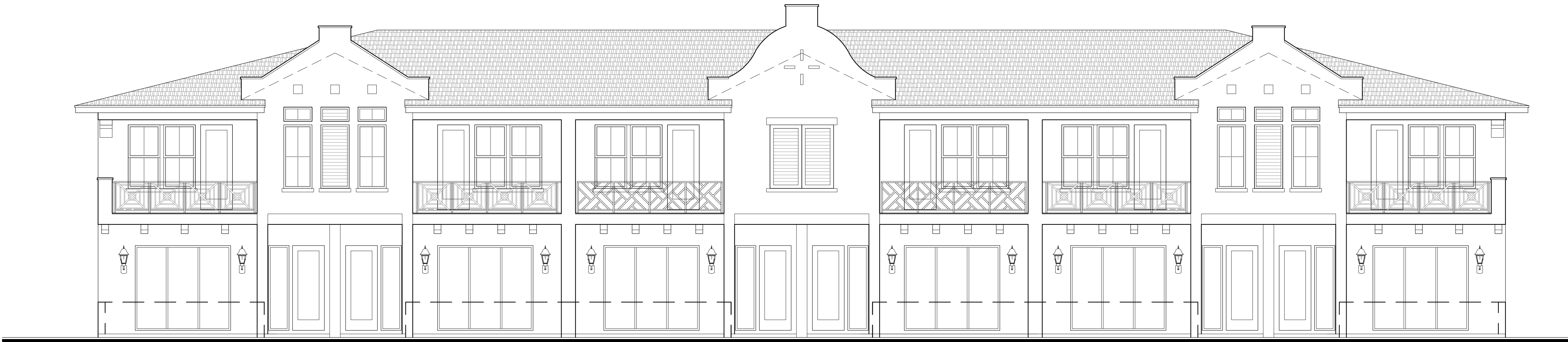
1 SIXPLEX - FRONT ELEVATION - (TYPE E) SCALE: 3/16" = 1'-0"
