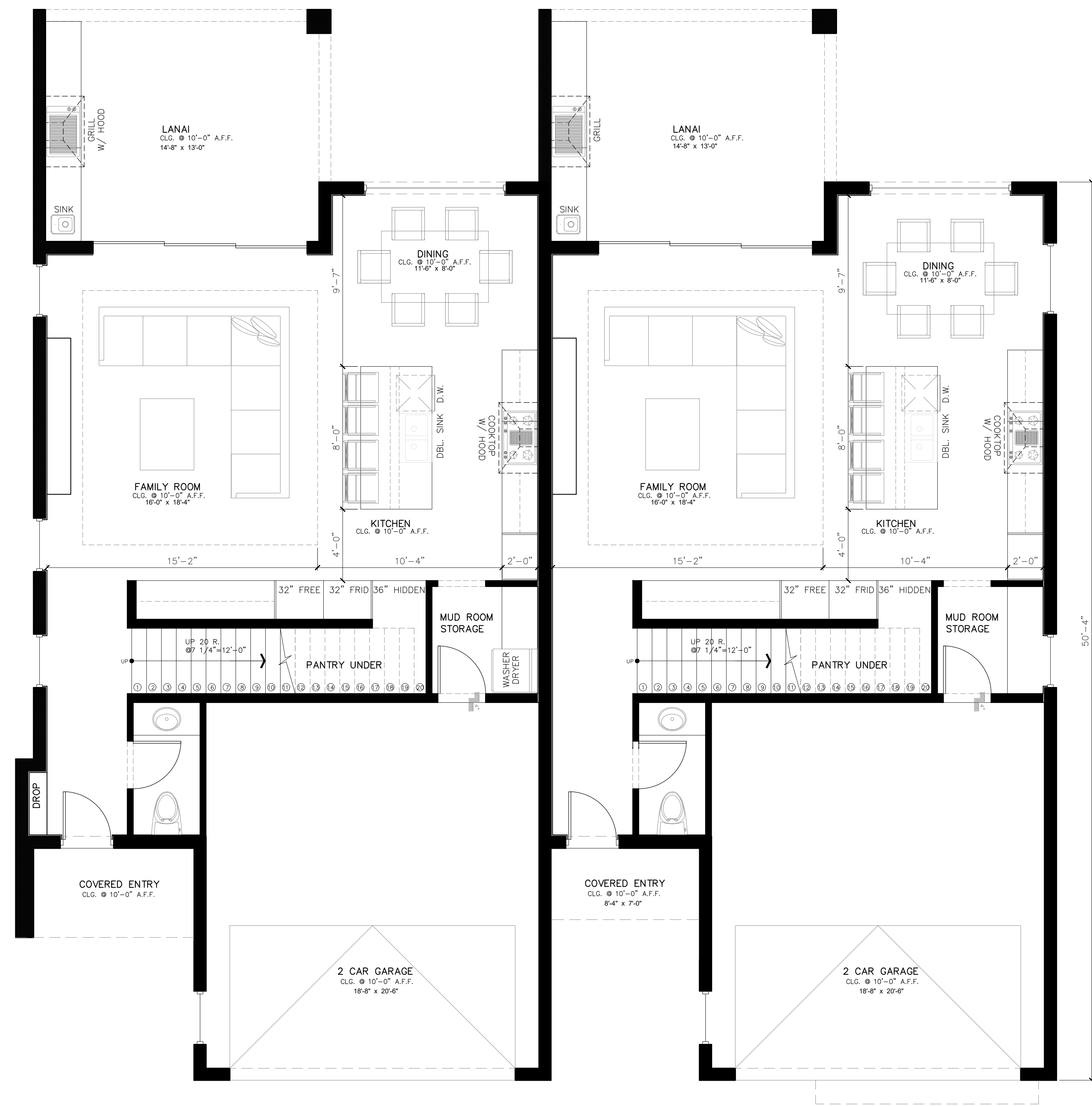
(BLOCK 2) 1ST DIM. FLOOR PLAN SCALE 1/4" = 1'
