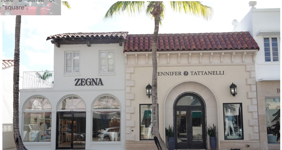
The building on the left ties the horizontal expression line into a balcony feature and suggests arched columns in the framing of its windows and doors. On the right, the one story building combines ornate pilasters, bracketed overhangs and a pitched roof accent which allows for a taller one-story building to feel less imposing.
