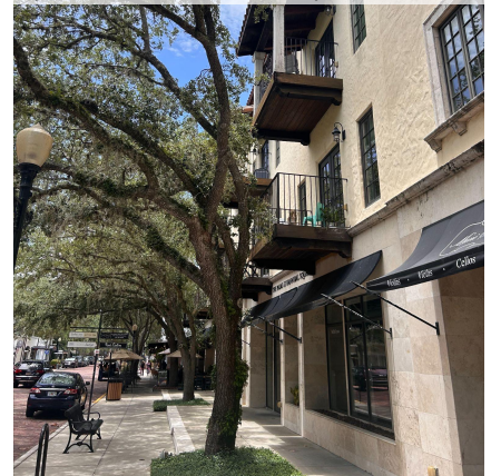
Cantilevered porches can add depth to a facade. A "heavier" base material on the first floor can emphasize pedestrian scale and allow for a more pronounced horizontal expression line.
