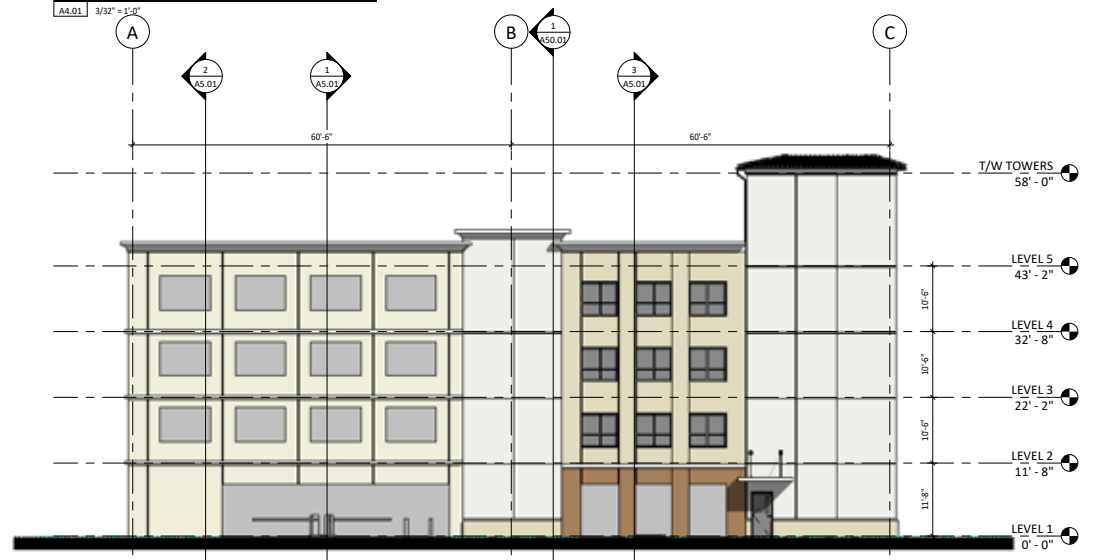
2 EAST BUILDING ELEVATION A4.01 3/32" = 1'-0"
