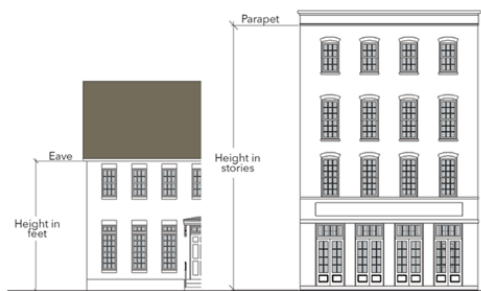
ILLUSTRATION 12-3-3.1. MEASURING BUILDING HEIGHT
