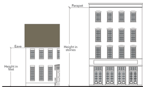
ILLUSTRATION 12-3-3.1. MEASURING BUILDING HEIGHT
