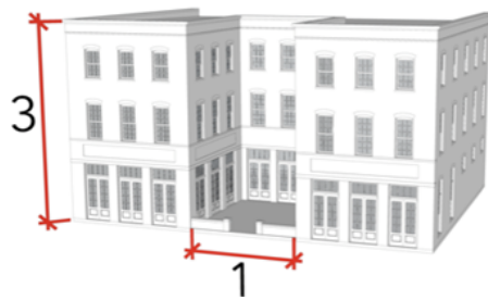
ILLUSTRATION 12-3-31.4. COURTYARD HEIGHT TO WIDTH RATIO MEASUREMENTS
