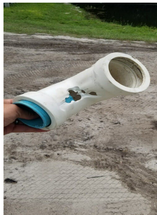
Old, worn and outdated irrigation equipment
