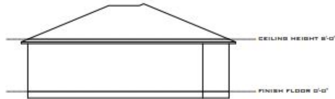
EXISTING SOUTH (GARAGE SIDE) ELEVATION
