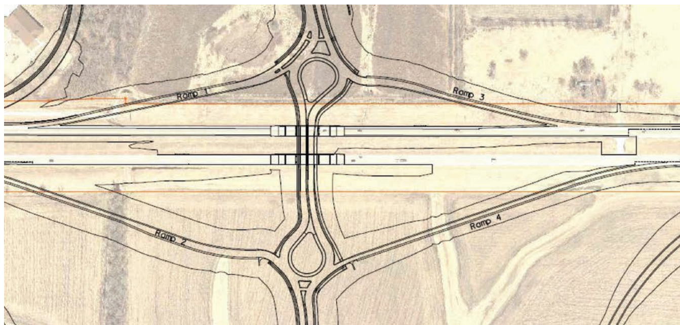
Figure 45. Roundabout interchange with teardrop-shaped central islands at each roundabout. (Photo source: Missouri DOT.)
