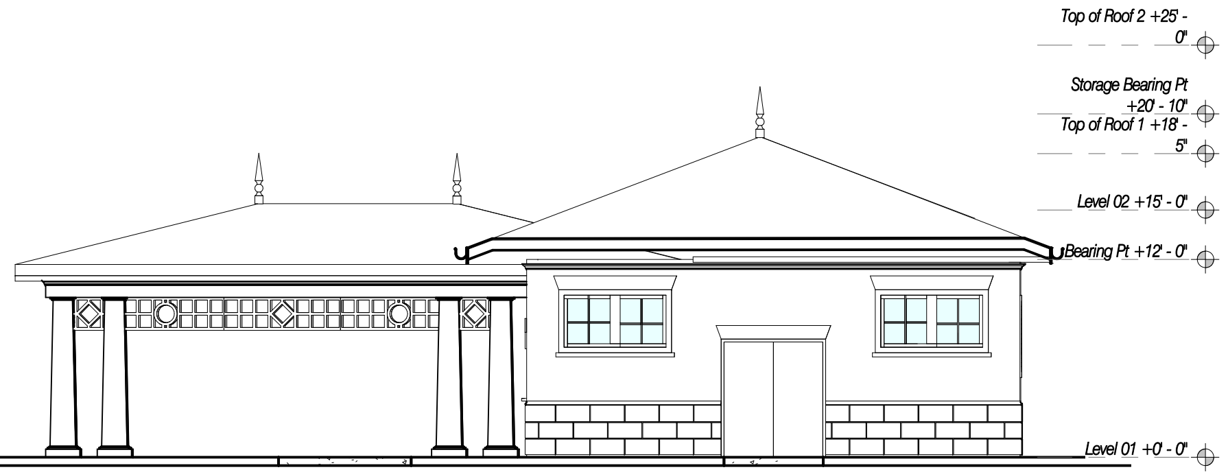
NORTHEAST ELEVATION Scale: 1/8" = 1'-0"
